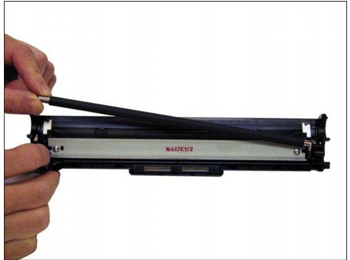
4. Remove the PCR. Clean with your preferred PCR cleaner and place aside.
