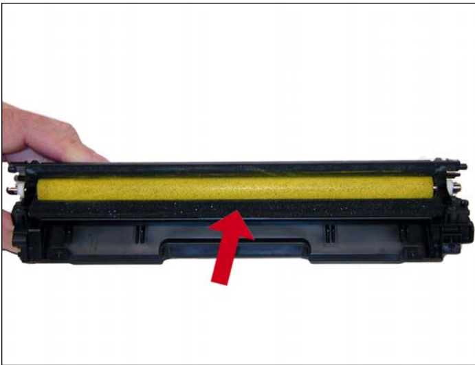
18. Clean the doctor blade foam seal. Install the doctor blade and two screws.
