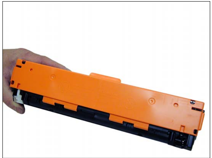
29. Install the drum cover on to the cartridge. Spread the two halves apart slightly so it fits properly.
