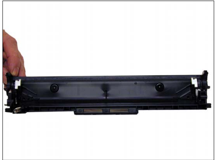
5. Remove the two screws and wiper blade.
