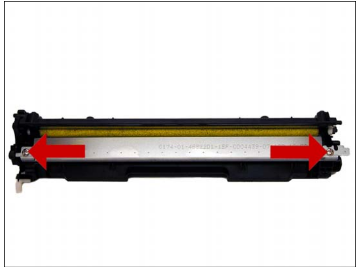
13. Remove the two screws and doctor blade.
