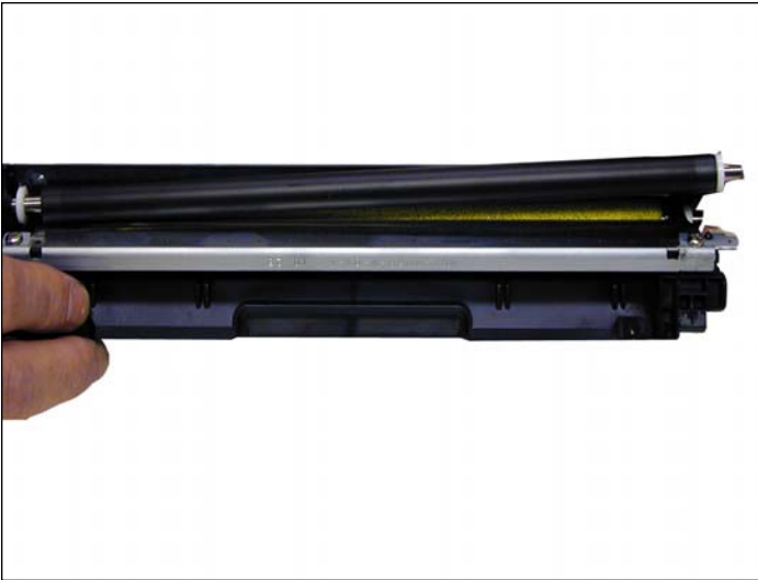
12. Slide the developer roller over and remove.
