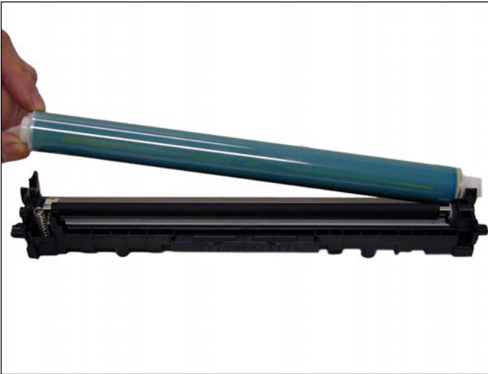
3. Flip the waste chamber upside down, and remove the drum.
