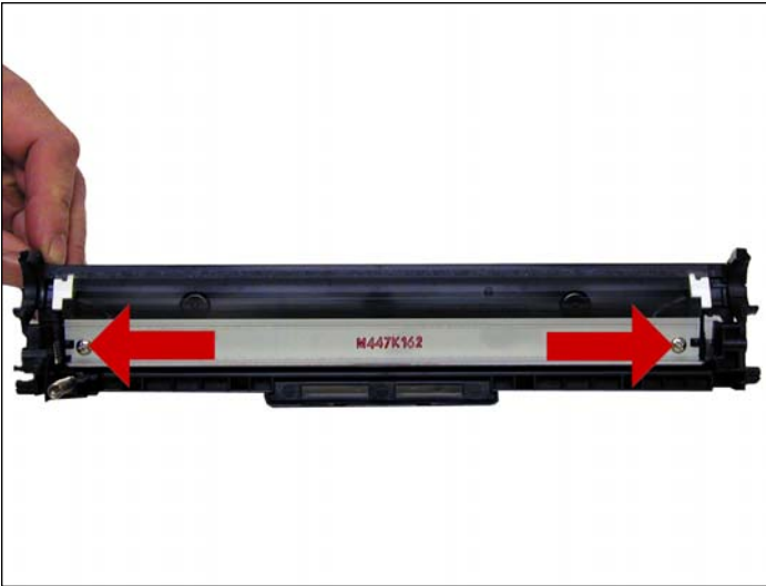
5. Remove the two screws and wiper blade.
